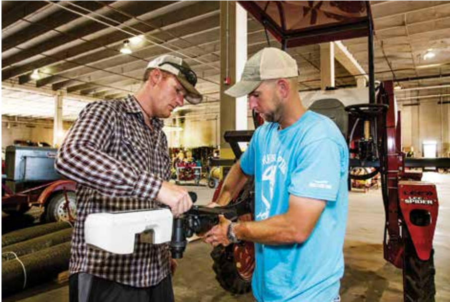
Assistant Professor Mark Newell, Ph.D., (left) and Josh Pittman install a remote sensor on a new vehicle that will measure taller forages.
