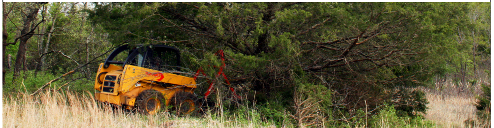
A skid loader equipped with a tree saw cutting down an eastern red-cedar that measured 22 inches in diameter at the ground level
